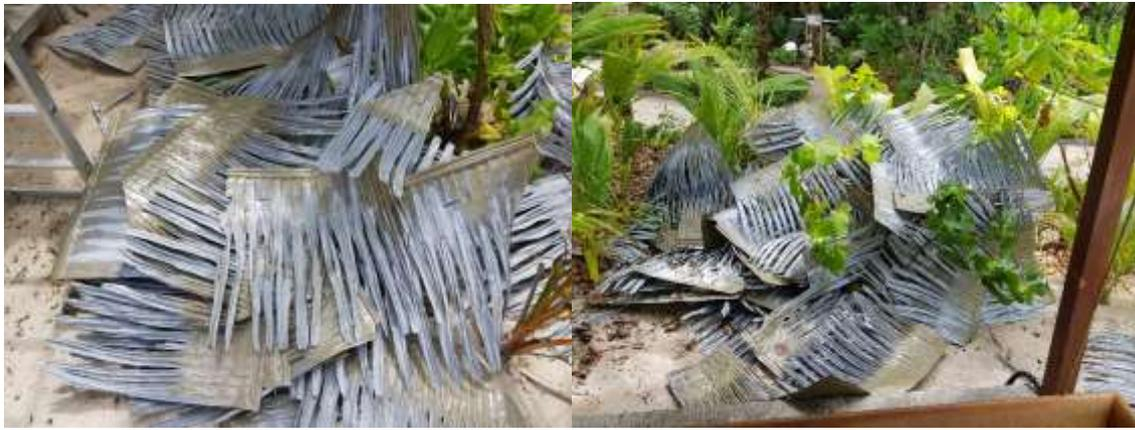
Synthetic tiles stripped from a resort roof shockingly **less than 2 years since installed as new**
